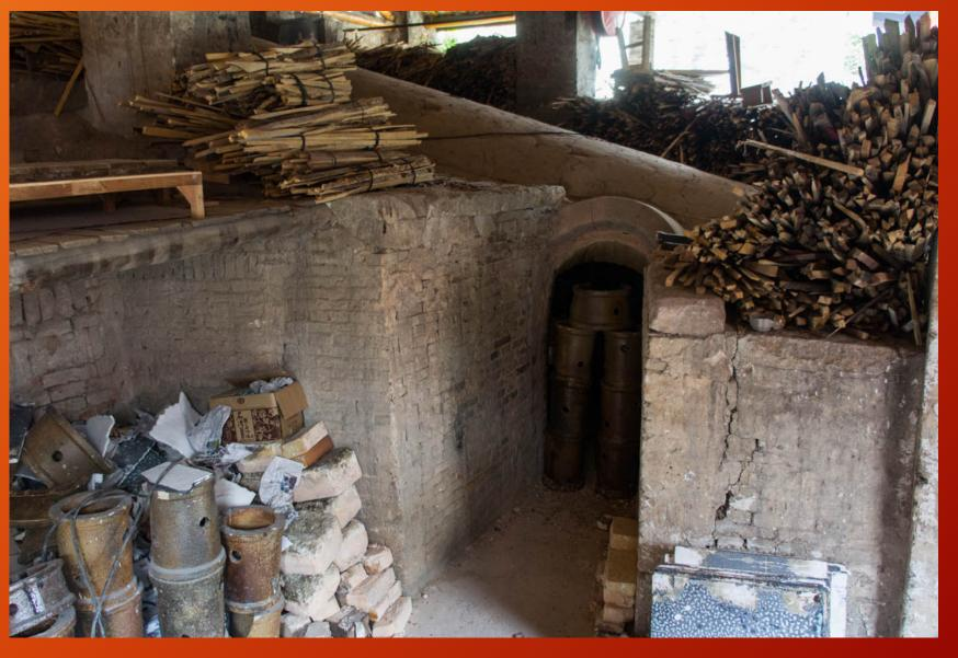
In this side entrance, located further up and on the opposite side of the kiln, can be clearly seen a number of refractory saggers into which the ceramic articles are placed. The external coloration of the saggers is caused by years of ash deposits falling onto the surface during repeated kiln firings.
